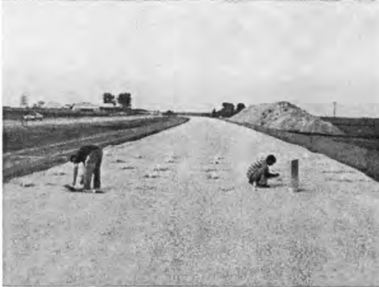
Figure 57 Photograph showing the process of measurements at grid points on US151 Test section
