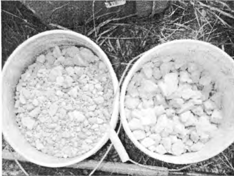
Figure 42. Quarry aggregate sample on left side and aggregate from trimmer on right side
