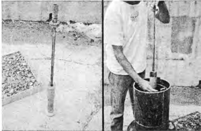
Figure B4. Marshall impact hammer (left) and compaction procedure (right)
